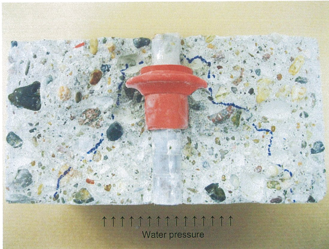
Fig. A2: Sample 1: anchor rod (ribbed steel \varnothing = 16 mm)
