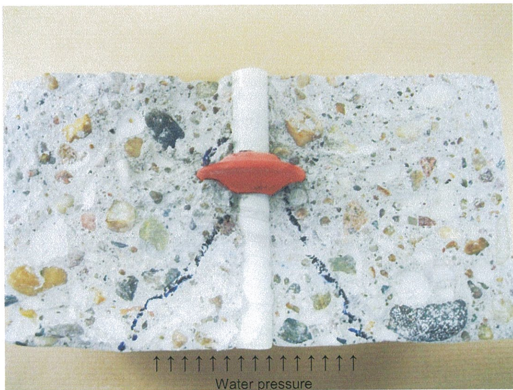
Fig. A3: Sample 2: glass-fibre rod (ribbed \varnothing = 14 mm)
